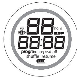
test pattern 2 (alternate segments activated)
